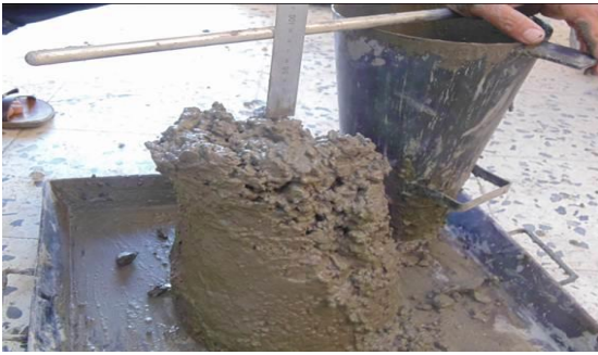
Figure 5. shows slump test
