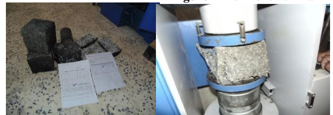
compressive strength test for a sample of concrete
