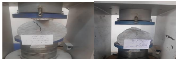
Figure 10. Shows indirect tensile tester of a sample of modified concrete.
